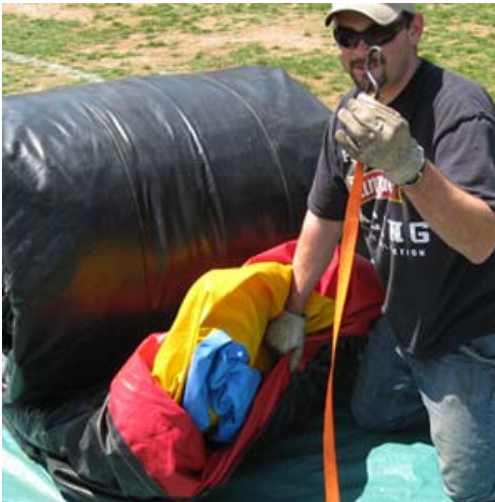
Step 6: Push straps 2-3 feet under the Inflatable (at Blower tube end) before rolling. Doing so now will keep you from lifting the entire roll later. (Ours have D-ring buckles, not "S" hooks).
