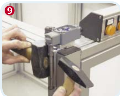
9 Lock by a plug pin the switch (plug pin supplied).
