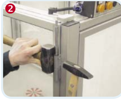
2 Lock by a plug pin the hinge to the shaft.
