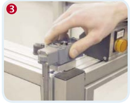
3 Insert the switch into the shaft.
