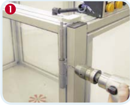
1 Drill the hinge and the shaft.
