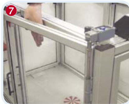
7 Check the operation point according to EN 294, if necessary adjust the operation point again (see fig. 6).
