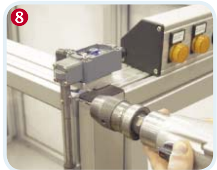
8 Drill the hinge shaft through one of the two holes in the shaft of the switch.
